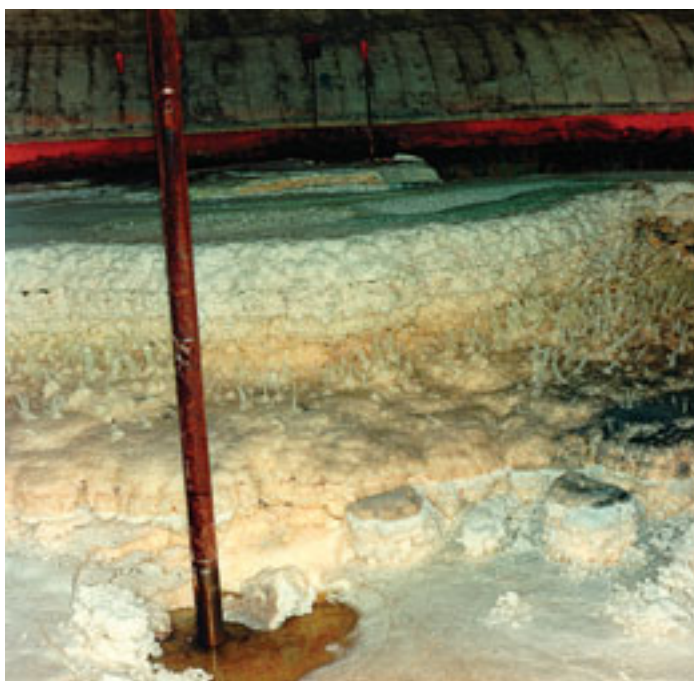
Before and after. Most of the waste inside Hanford's older single-shell tanks is in the form of saltcake, with the consistency of wet beach sand, and sludge, which looks like fine mud and dries very hard. After being vitrified, it looks far more homogenous (see inset).
